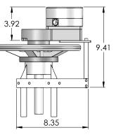
Hanbay's G-Stage mounting kit adapts to any gate valve up to 6" in size. Reduce open and close time with this 12-24VDC compact actuator. It also works on rising/non-rising gate valve stems.
