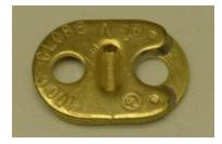
**Thermal Cutoff:** This UL approved part is found inside the enclosure, connected to the circuit board. When overheated it will sever the electrical connection, allowing the actuator to close itself via spring return.
