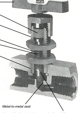
Integral back-seated stem standard on globe patterns. Exclusive safety feature prevents accidental removal of stem
