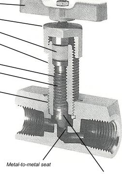
Integral back-seated stem standard on globe patterns. Exclusive safety feature prevents accidental removal of stem
