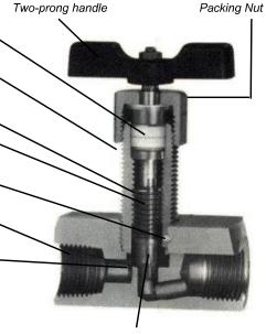
Integral back-seated stem standard on globe patterns. Exclusive safety feature prevents accidental removal of stem and eliminates possibility of stem blowout
