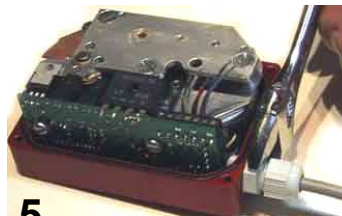
5.- Put the liquid tight fitting back and tighten (lightly with tool)
