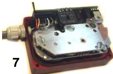
4.- Insert the cable into the actuator base
