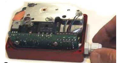
6.- Hand tighten the liquid tight fitting to establish seal
