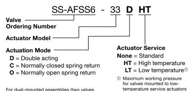
For dual-mounted assemblies (two valves mounted to one actuator), add **DM** to the ordering number. Example: SS-AFSS6-33DHT**DM**
