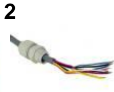
2.- The cable has to be stripped of its jacket for 2 inches (50mm) and the wires need 1/8" (3mm) stripped ends.
