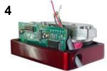
4.- Carefully insert the cable into the actuator base. Mind the red motor cable and its plug into the board. Moving the plug out of its fully inserted position may cause malfunction of the actuator.
