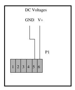
Locate the correct connection terminals as shown in the picture to the left then connect according to the connection schematics above.
