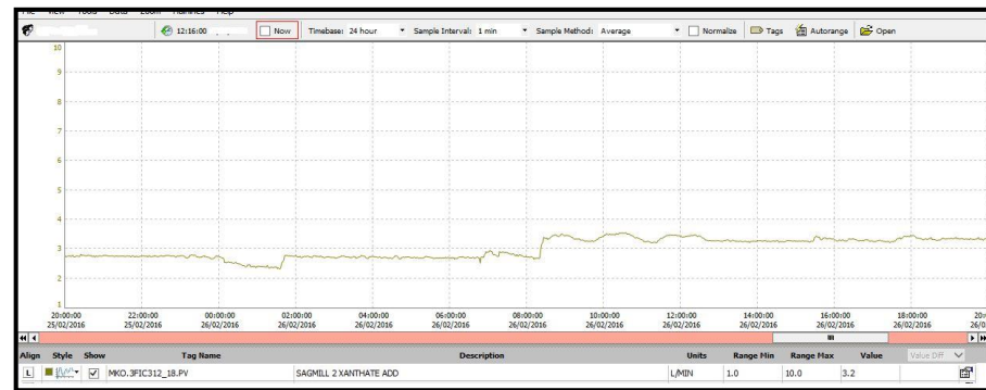
A trend screenshot from the DCS of the reagent process variable (with no set-point changes) when the existing GEMU valve was used.
